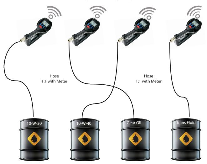
Up to 8 Fluid Types and 8 Tanks per Keypad
